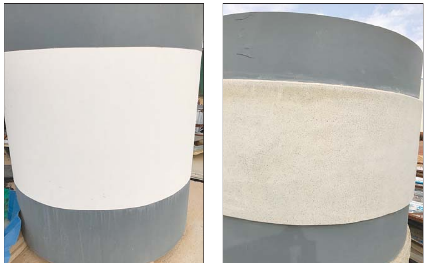
Fig. 2. Mockup of intumescent and cementitious
